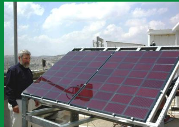
Outdoor testing of DSC tiles by 3GSolar in Jerusalem 2005- 2008
